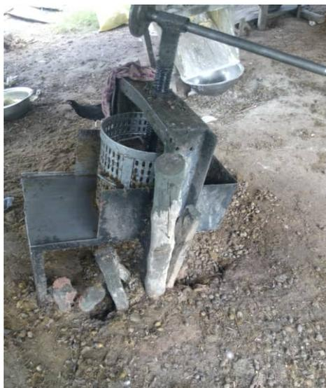
Plate: A curb press used by processors at Obareren, Ovia North East LGA Edo State
