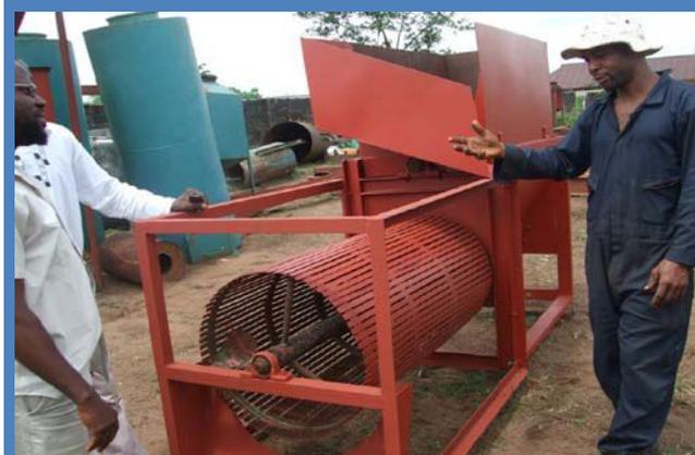
PIND is working to facilitate the introduction of improved palm oil processing equipment. The whole bunch stripper pictured above will enable millers to process palm oil more efficiently and thereby generate more income.
