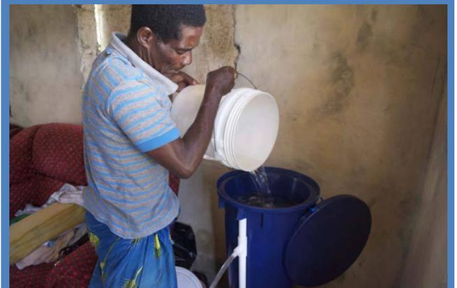
A community member demonstrating how to use the bio-sand filter. Unsafe drinking water is poured into the container and filtrated.
