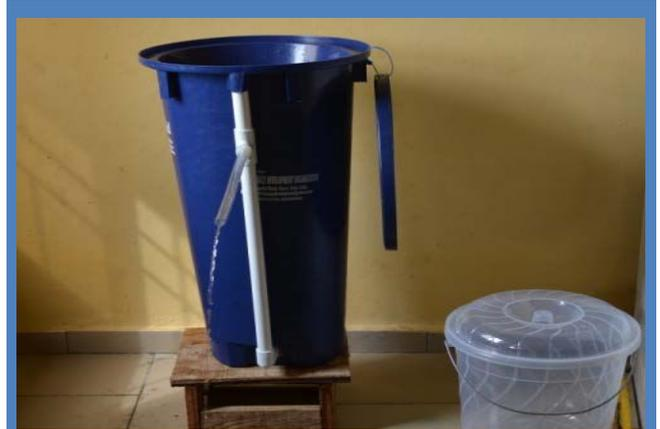
The bio-sand filter is an example of an appropriate technology. It is inexpensive to build and is 99% effective at removing pathogens from water. This simple and effective device can make water from a shallow dug well safe for human consumption and produce enough clean water each day for a family.
