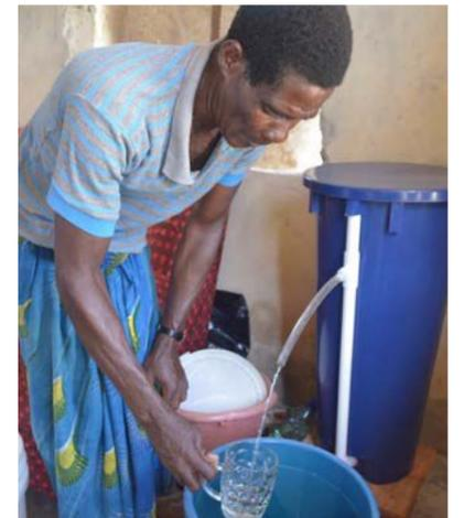
NDPI's Appropriate Technology Enabled Development (ATED) program introduces simple, new technological solutions for development challenges in the region, such as the bio-sand filter shown above, which is a low-cost means of producing safe drinking water for households.
