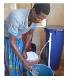
NDPI's Appropriate Technology Enabled Development (ATED) program introduces simple, new technological solutions for development challenges in the region, such as the bio-sand filter shown above, which is a low-cost means of producing safe drinking water for households.
