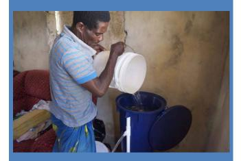
A community member demonstrating how to use the bio-sand filter. Unsafe drinking water is poured into the container and filtrated.
